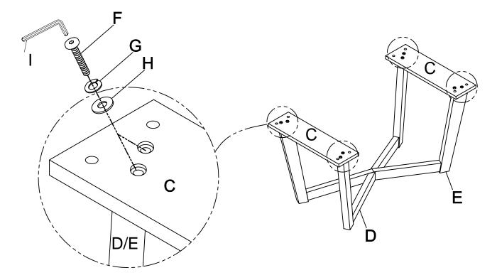
2 Use Allen Bolt(F) Lock Washer(G) and Flat Washer(H) on holes of Leg Down(D). Turn the Allen Key(I) in Allen Bolt(F).
