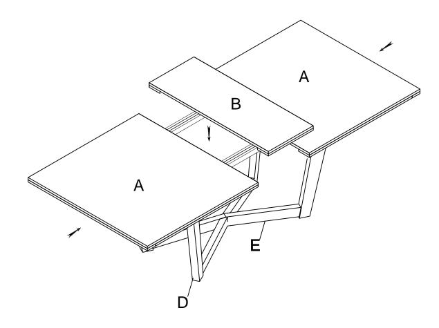
7 Lock the Leaf(B) by using Sash Lock.
