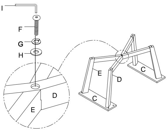
**3** Attached Mounting Plate(C) to the Table Top(A). Use Allen Bolt(F) Lock Washer(G) and Flat Washer(H) on holes of Table Top(A). Turn the Allen Key(I) in Allen Bolt(F).
