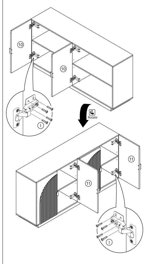
When the clearance of the door is uneven, Adjust the cabinet door according to the figure. If you still have trouble while adjusting the door, please contact us.
