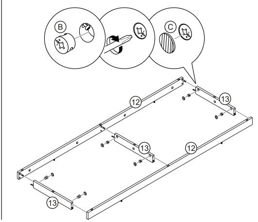
Assemble the base assembly to the underside of the bottom panel (2).
