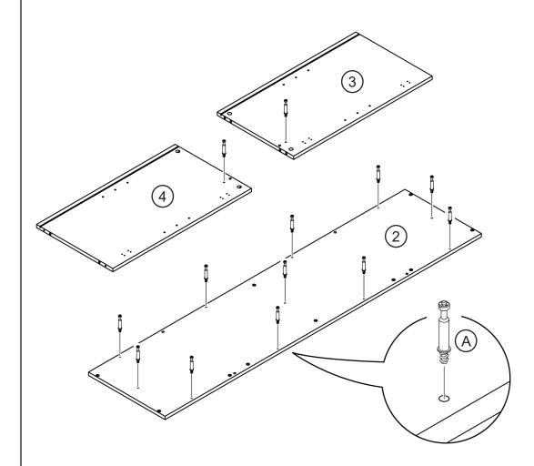
Attach cam bolts to both sides of the medial panel (5).
