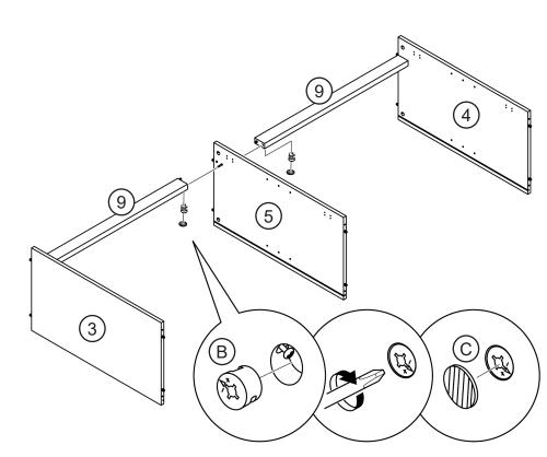
Assemble the medial panel (5) between the two crossbars (9).
