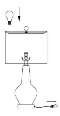
Step2 Insert the bulb(G) into the socket(C).
