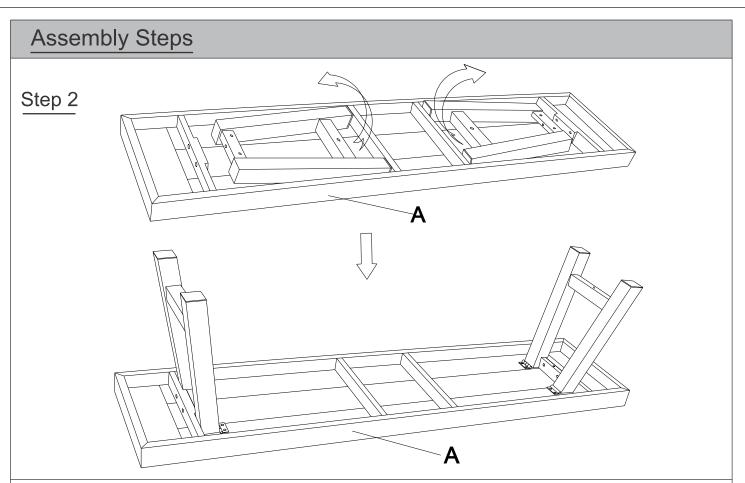
Place the Bench (A) with the fabric face skywards onto a clean, soft surface to avoid any scratches or damages to the product.
