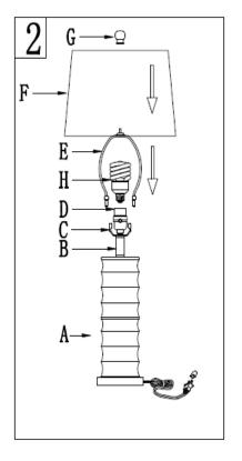
Step 1 Screw the Neck (B) onto the Lamp base (A) Be careful not to twist the power cord and tighten securely Step2
