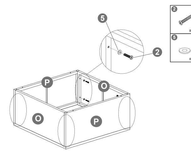
(Tips: after all holes are aligned, then fixed to 100%)
