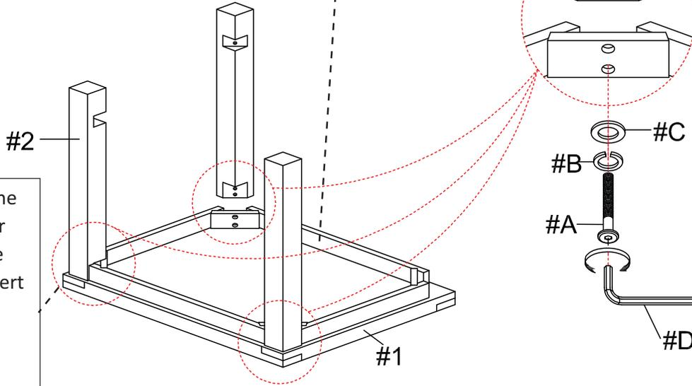
3. Align the top of the legs (#2) to corner holes on the table top (#1). Then insert 2 bolt assemblies into each corner and secure using the Allen wrench.
