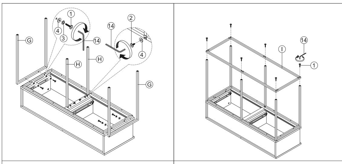
STEP 5 ATTACH LEG FRAMES AND CENTER LEGS TO UNIT USING 30 MM BOLTS, 15 MM BOLTS, SPRING WASHERS AND FLAT WASHERS. TURN BOLTS USING ALLEN KEY.
