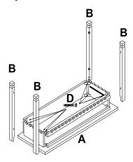
**Step 4**Attach Bottom (C) to Post (B) using 4-45MM Hex Bolts (D). **Note: TIGHTEN ALL BOLTS AT THIS TIME!** Attach wooden knob to outside of drawer front. Insert the Drawer in to the Top Assembly.
