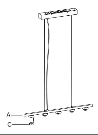
Put Glass Shade (B) on the Light Body (A) and put the Accessory (C) back to tight the Glass Shade (B).
