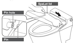
2 Open the pin hole on the right side of the SpaLet lid outwards and then align the pin with the pin hole to attach the SpaLet lid.
