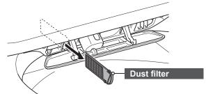
**3** Wash the dust filter to remove dust and dirt.
