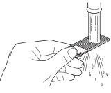
4 Allow the dust filter to dry and then reinstall.
