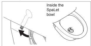
4 Once the waste has been flushed, turn the red flushing lever toward you again and hold it in this position for approximately 5 seconds.
