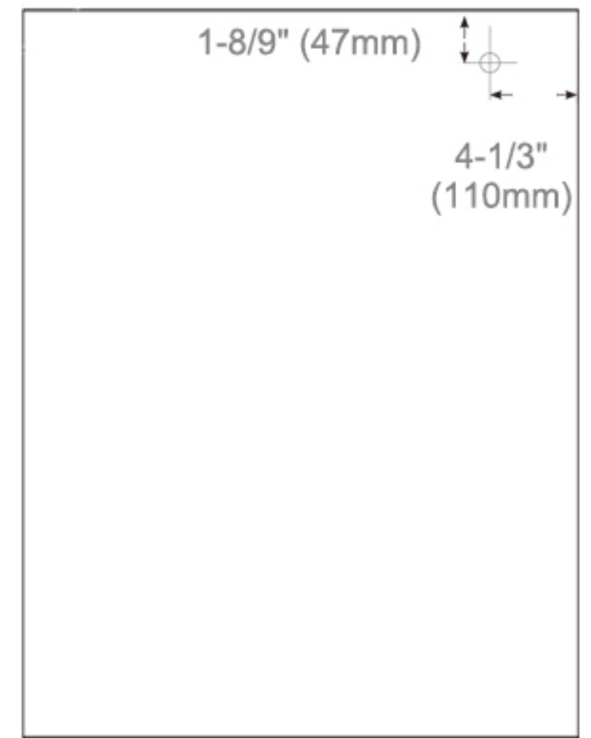
Back of Cabinet - Wire Access Location
