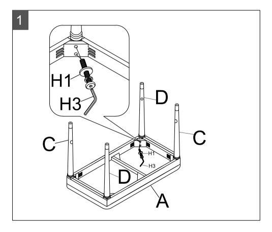
Step 1: Attach 4\*legs (C, D) with cushion (A) .Use allen key (H3) to lock with 8\*bolts (H1).
