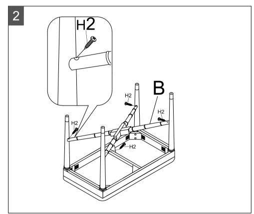
Step 2: Attach set of cross bar (B) with leg (C). Use 4\*crew (H2) to lock.
