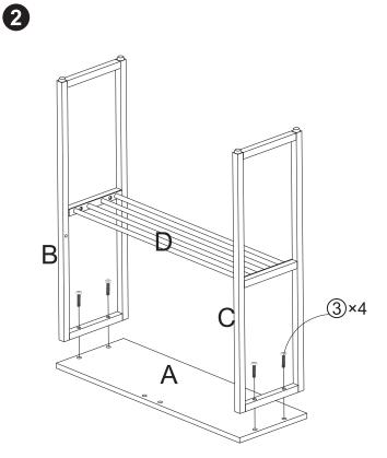
Screw (3) through the holes in (B) and (C) respectively into (A).
