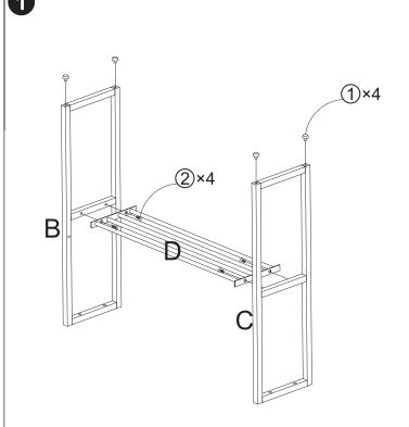
Screw (2) into (B) and (C) through the holes in (D). Screw (1) into the holes of (B) and (C) respectively.
