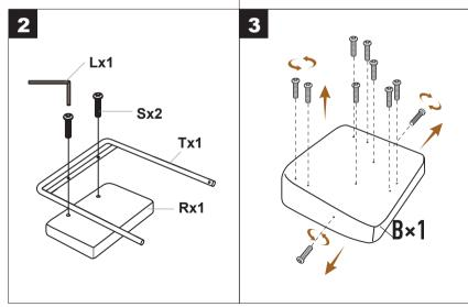
**Note:** All screws havebeenpreassembled to the accessories Please remove them from the accessories before assembling
