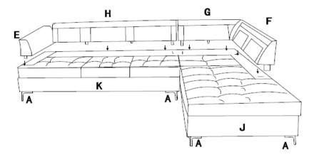
**Step 3** Aligh the entire back cushions to the back rest, attach to the Velcro, adjust and fix it properly.
