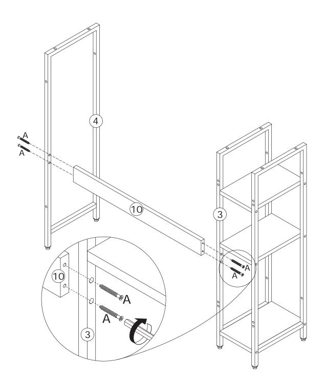
Fix part 3 and 4 to board 10 with screw(A) as shown.
