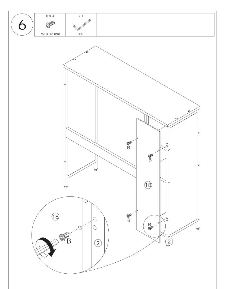
Fix board 18 to part 2 and 3 with screw(B) as shown.
