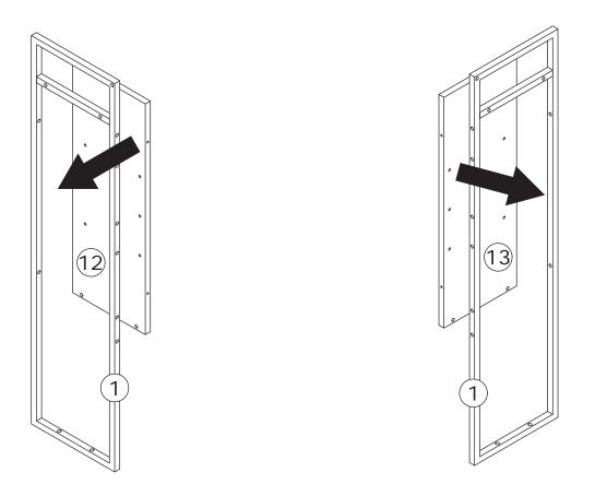
Fix board 12 and 13 to part 1 with screw(A) as shown.
