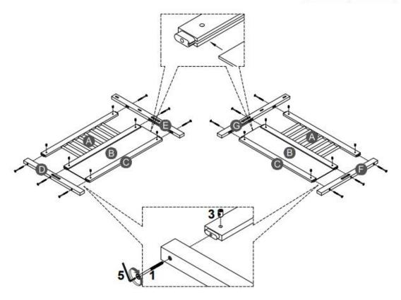
Note:Part 3 will face up with the "x" mark on it, otherwise it cannot be tightened
