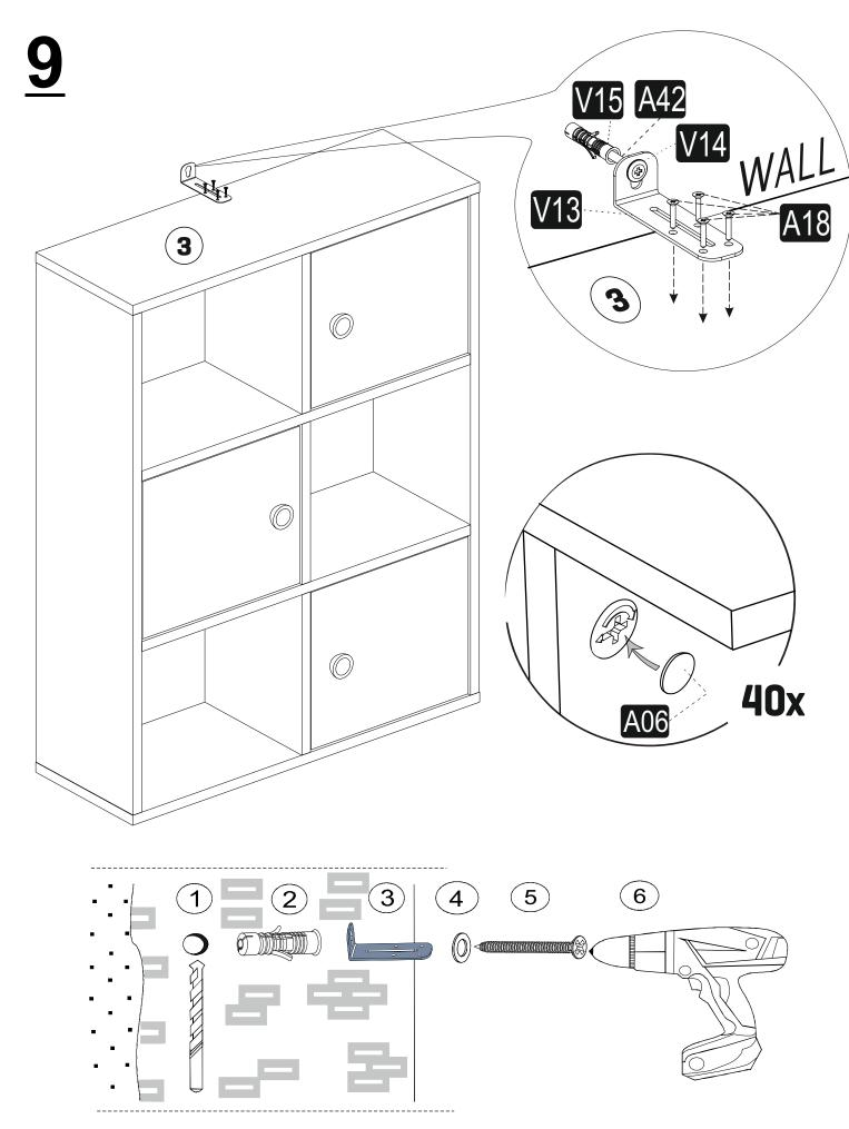
Check the Wall type before installation of dowel. Wall is drilled with equal diameter of dowel.(08mm) Universal Plastic Dowel provides the general purpose usage. Requires two stages assembly.
