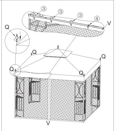
Step8:Insert four Part Q to four corners of the frame,then turn it to be tight. Use three Part3 and one Part4 per side to hang the netting on the frame.
