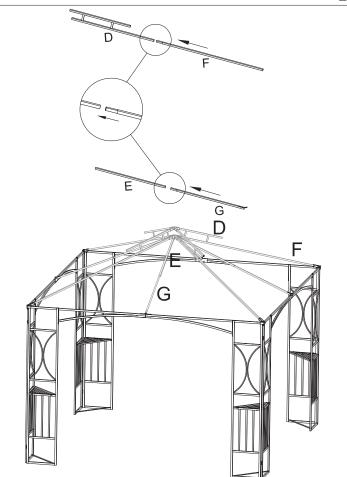
Step3:Insert small head of Part F to the long side of Part D,insert small head of Part G to Part E.Please note:Part E is a short pole,Part F is a long pole.
