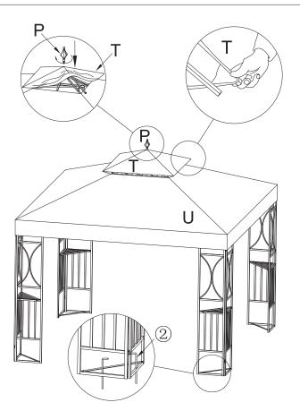
Step7:Install Part T,U on the frame and expand them.Make the four corners of the frame covered fully.Then put the top poles into the corner pockets of Part T.Insert Part P to Part K,turn it.Insert Part② through the bottom of Part A to the ground.
