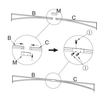
Step2:Put Part B and Part C together,and insert Part M to the side of Part B and C.Use three Screw① to tighten them.
