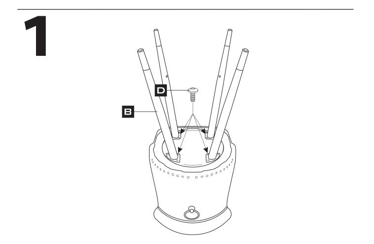
Assemble all parts and bolts loosely during assembly
