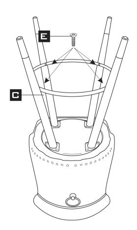
Assemble all parts and bolts loosely during assembly
