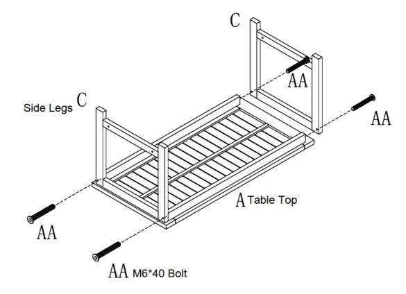
Attach the (2) Side Legs (Part C) to the underside of the Table Top (Part A) using (4) M6\*40 Bolts (Part AA).
