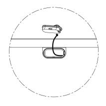
4 Align the sensor with the opening on the fixture and snap into place.
