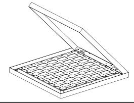
f installating sensor, lay the fixture face up on a flat surface. Using a pry tool or small screwdriver, remove the sensor socket cover and remove the wire from the back of the cover. Otherwise skip to step 5.
