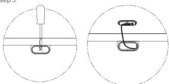
Plug the wiring into the socket on the back of the motion sensor.
