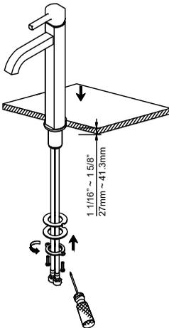
Install the faucet through the 1-3/8" predrilled hole in the countertop. Attach rubber washer (4A), metal washer (4B), mounting nut (4C), and mounting screws (4D) on the threaded mounting pipe. Tighten the mounting nut (4C) until snug. Tighten screws (4D) on the mounting nut (4C) with a Phillips head screwdriver until snug.
