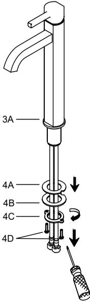
Remove rubber washer (4A), metal washer (4B), mounting nut (4C), and mounting screws (4D). Keep the base trim ring (3A) and rubber washer (3B) on the base of the faucet.
