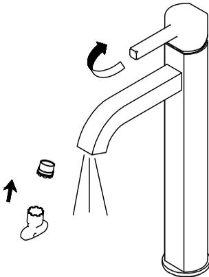
After installing the faucet, remove the aerator (2) with the included aerator key (6). Turn on the water to remove any leftover debris, then reassemble the aerator (2).
