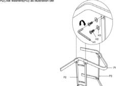
Step 2.Using bolts (H5), lock washers (H6), flat washers (H7), attach legs (P1) to chair (P4). Tighten bolts (H5) with allen wrench (H4) as illustration below.
