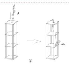
Step 8: Pass the plug, butterfly nut, and washer through the top panel, and drop the pull chain through the square hole.
