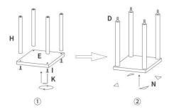
Step 1: Use the hex wrench to fix the bottom panel and the iron poles (4PcS) firmly with No.1 screw(4 PCS).
