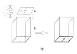
Step 9: Put the bracket into the lampshade from top to bottom and fix the bracket with the buckle. Where the crossbar intersects with the C-shaped iron sheet, the protruding part of the crossbar faces downwards.
