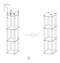
Step 7: Similar to step 6 screw on the iron poles, and then fix the top panel on the poles firmly with the No.1 screw(4PCS) via hex wrench.
