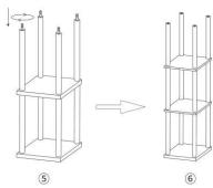
Step 5: Rotate No.2 screw(4PCS) and fix them to the top of the iron poles. Step 6: Pass the other middle panel through No. 2 screws and place it on the iron poles.
