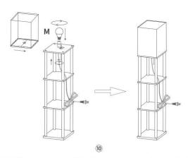
Step 10: Lift the lamp cap slightly, let the wire pass through the C-shaped notch of the lower bracket. Press the lamp socket firmly against the bracket and then tighten the wing nut under the lamp cap to fix the lamp cap and lampshade. Please note that the notch is facing the pull chain so as not to get caught in the pull chain.
