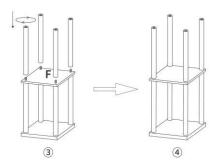
Step 3: Put the middle panel on the iron poles through No.2 screw. Step 4: Tighten the iron poles and fix them on the middle panel.
