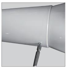
Remove the screw on the air duct (A), and separate the air duct (A) from the main body of the dryer (C).
