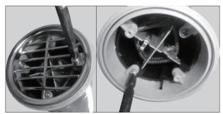
4). Unscrew the vent cover from the front of the air duct (A).
