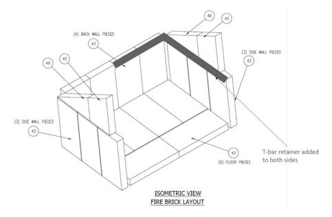
3. Finally, the T-bar retainer pieces (2) should be installed on both sides in order to keep the bricks in place.
