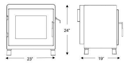
All clearances, side, corner, and back, are measured from the largest dimensions.
