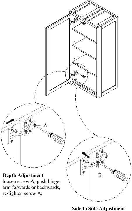
Side to Side Adjustment loosen screw B, adjust gap with screw B and re-tighten Screw B.
