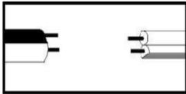
\*Note: When parallel wire ( SPT I & SPT II ) is used. The neutral wire is square shaped and ridged and the hot wire will be round in shape and smooth. (See Illustration on left.)
