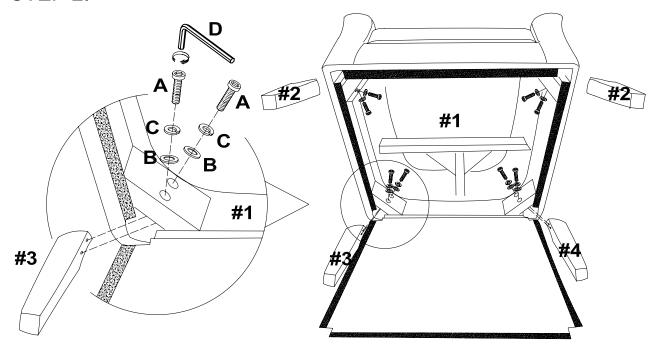
imporant: with insert nut head exposed opposite to get the leg being assembled in correct shape and good safe structure
