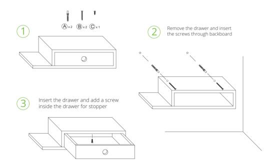
**Wall fixings:** Because of the variety of different wall types, We cannot provide you with exact fixing you will need to fix this product to the wall. You must first identify the type of the wall you intend to fix product onto and then contact your local hardware store to get the appropriate fixings.
