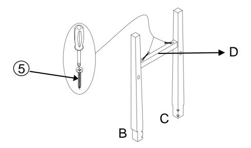
Insert the Short Side Rail (D) into the oval holes of Legs (B,C) forming an 'H' frame by using Screws (5) and Screwdriver as shown above.
