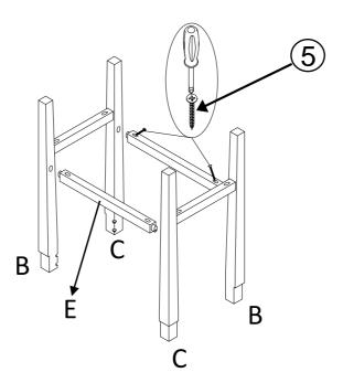
Insert the Long Side Rails (E) into the oval holes of the 'H' leg frame in Step 2 by using Screws (⑤) and Screwdriver as shown above.
