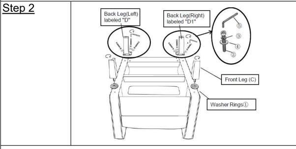
Install the Front Leg(C) and Back Leg(Left&Right) into the bottom of theChair Base Body(B) by placing a Washer Ring (①)Bolt(②)Spring WasherRing(③)Flat Washer Ring(④) with Allen Key(⑤)onto the threaded stem.And then insert the threaded Stem into the threaded Mounting Position ateach Corner of the Bottom of the Chair.
