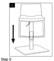
Align the column (D) onto middle of the frame as pictured. Place the assembled seat onto the base Use allen key "H4" to lock the 4 screws "H2".
