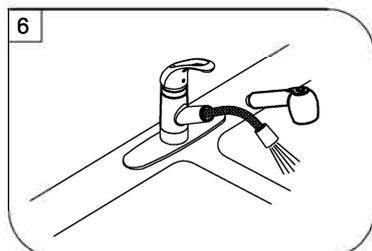
**Important:** After installation is completed. Turn on water supply and allow both hot and cold water to run for at least one minute each. Check all connections for leaks. Re-tighten if necessary, but do not overtighten.Reinstall Spray head. Your new faucet is now ready to use.
