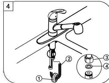
Install Weights(1) onto spray hose (2).Connect hose to outlet tube(3) and tighten. Do not overtighten.
