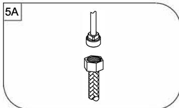
(A) Stainless Steel Braided Faucet Supply Tubes: This is the simplest of all installations. If you are using stainless steel braided faucet supply tubes, this faucet requires one end of the supply tube to have a 1/2" female IPS connection. The other end of this supply tube must match the thread on the water supply fittings or shut off valve under your sink. Once you have identified the required tube, carefully follow the manufacturer's installations instructions for each tube
