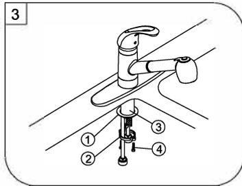
Assemble Washer(1),and thread Mounting Nut(2) onto Shank(3) from underside of sink.Handtighten.Secure Locking Screws(4) on Mounting Nut(2) and tighten Locking Screws(4) using screw driver.
