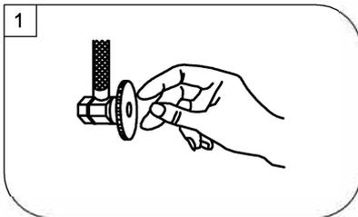
Shut off water supplies. Remove old faucet. Clean sink surface in preparation for new faucet.
