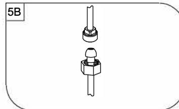
(B) Ball Nose Flexible Supplies: If you are using ball-nose flexible supplies to connect the faucet to water supply lines: Slip coupling nut behind ball-nose of flexible supply tube. Ball nose coupling will go partially into IPS shank or fitting. Tighten coupling nut (DO NOT OVER TIGHTEN). Install opposite end according to manufacturer's instructions for both tubes.
