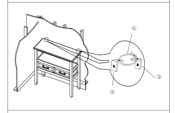
**C**: Move the Cabinet against the wall. Then pull the Cabinet Restraint Strap(④) through two Metal Brackets(③) one by one, lock tight the Cabinet Restraint Strap(④), as shown above.
