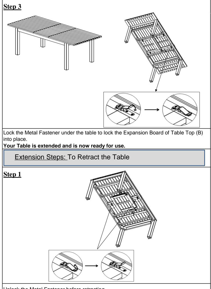
Unlock the Metal Fastener before retracting.
