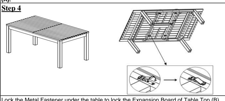
Lock the Metal Fastener under the table to lock the Expansion Board of Table Top (B) into place.
