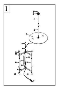
Step 1 Make sure all parts could be aligned before assemble Do not rotate lamp body too hard avoid base screw broken Let tube(A1) go through Fork frame(E1), and screw tube(B1) onto tube(A1)
