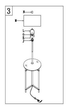
Step 3 Insert the Harp (L) into the Saddle (J). Put the shade(M) on the Harp(L), then tighten the Finial (N) into the Harp (L) Insert the bulb(O) into the socket(K).
