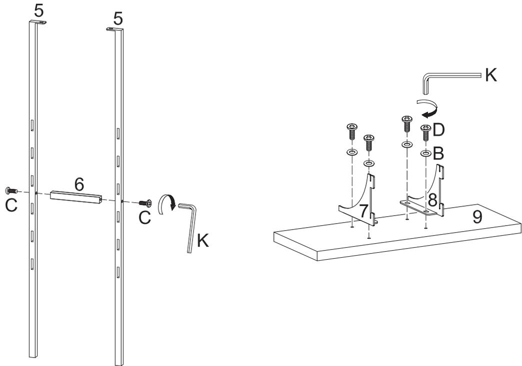
Attach shelf racks (5) to shelf crossbar (6) using large bolts (C). Build each shelf by attaching shelf supports (7,8) to shelf top (9) using small bolts (D) and washers (B).
