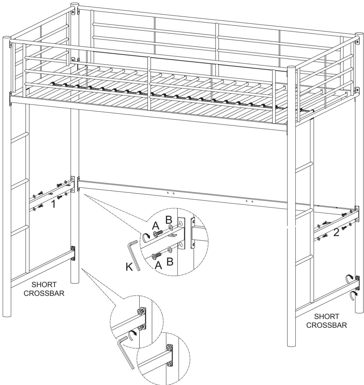
Attach crossbars (1,2) to the bunk bed frame using medium bolts (A) and washers (B). Retighten the bolts that secure the short crossbars.
