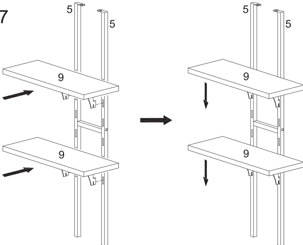
Attach the assembled shelves from Step 6 to shelf racks (5) by inserting them in at the desired height and gently pushing down to lock in place.
