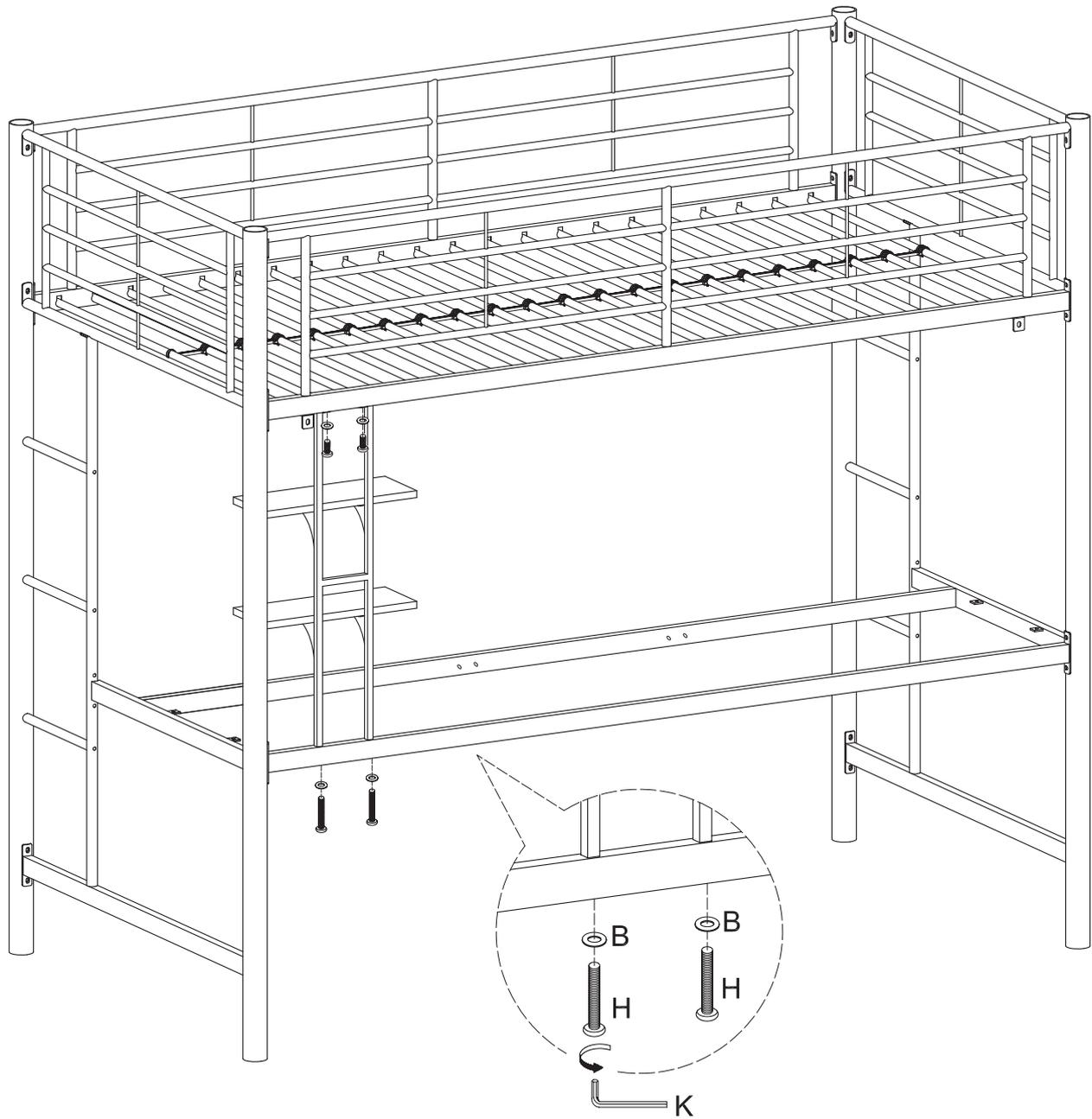
Attach the shelf assembly from Step 7 to the bunk bed frame using extra-large bolts (H) and washers (B).
