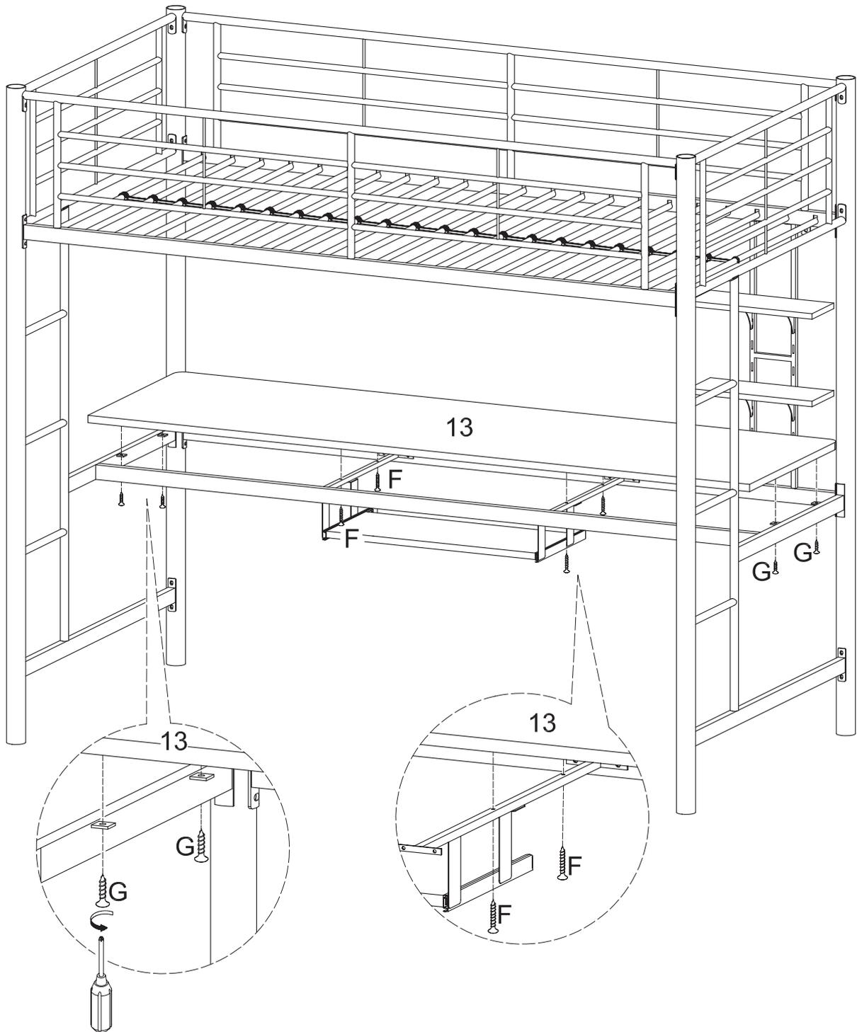
Attach the desk top (13) to the bunk bed frame using medium screws (G) on either end, and large screws (F) at the keyboard tray assembly.
