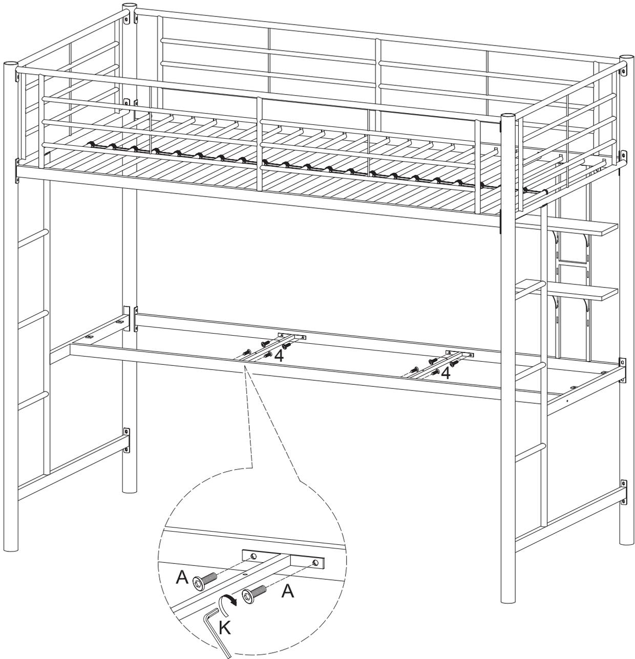
Attach desk crossbars (4) to the bunk bed frame using medium bolts (A).
