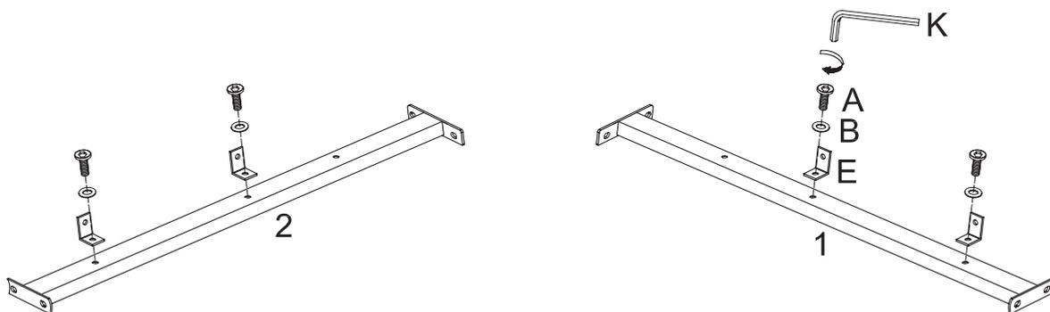
Attach angle brackets (E) to crossbars (1,2) using medium bolts (A) and washers (B).
