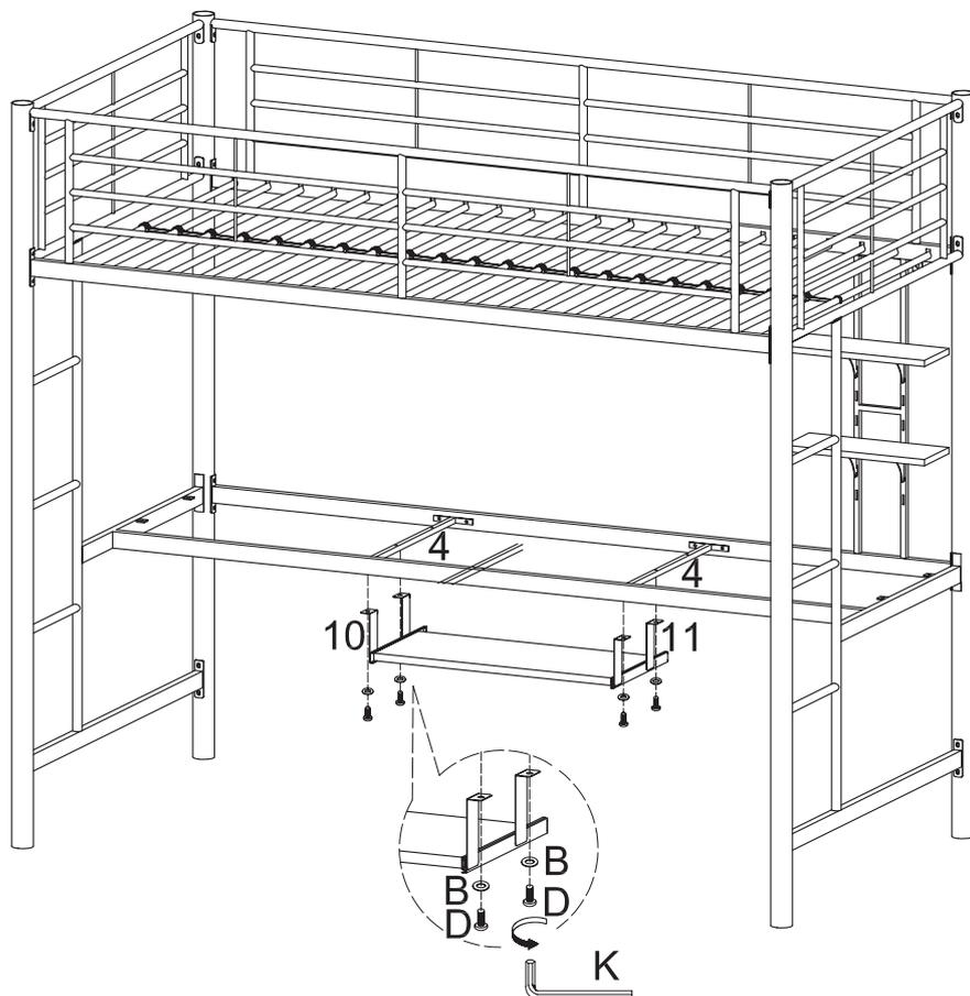
Attach the keyboard assembly from Step 10 to crossbars (4) using small bolts (D) and washers (B).
