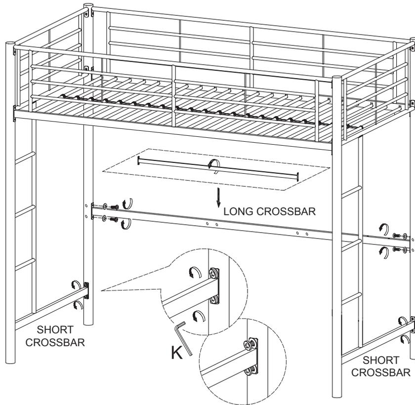
Remove the long crossbar from the bunk bed frame and turn it over so the screw holes are facing forward. Reattach the long crossbar to the bunk bed frame using the bolts and washers from Step 1. Loosen, but do not remove the bolts that anchor the short crossbars to the bunk bed frame.
