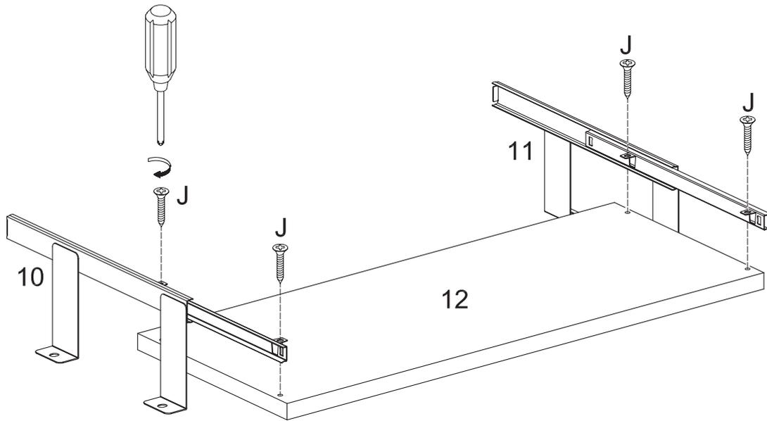
Attach keyboard sliders (10,11) to keyboard tray (12) using small screws (J).
