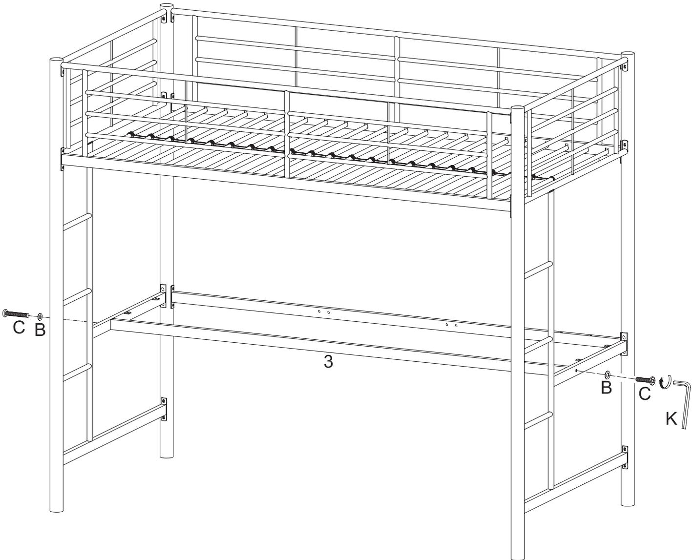
Attach crossbar (3) to the bunk bed frame using large bolts (C) and washers (B).
