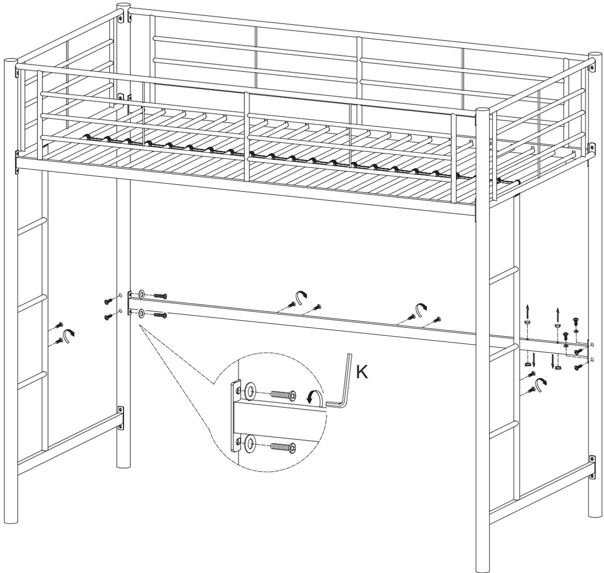
Remove the bolts, washers and plastic plugs shown above from the bunk bed frame.
