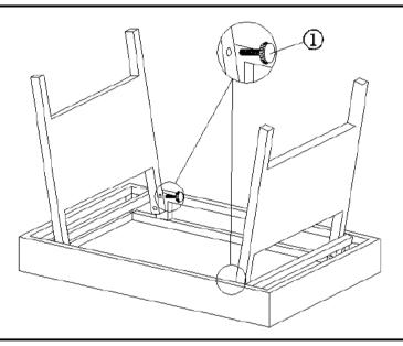
Attach the Table Legs to the support bar on the Table Top using Bolt(1) as pictured.
