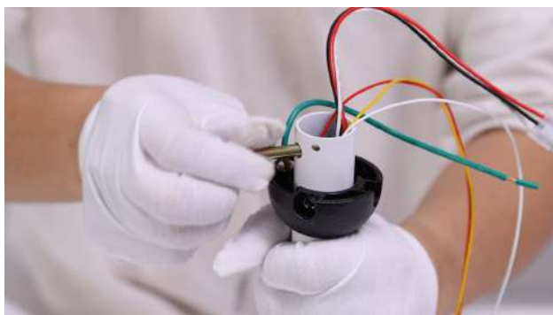
25. Connect the wire from the ceiling fan to the receiver (Red, White and Black wires)
