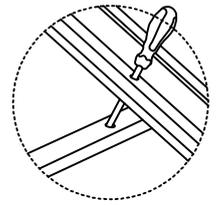
If the screw hole is out of alignment, insert it with a screwdriver and correct it
