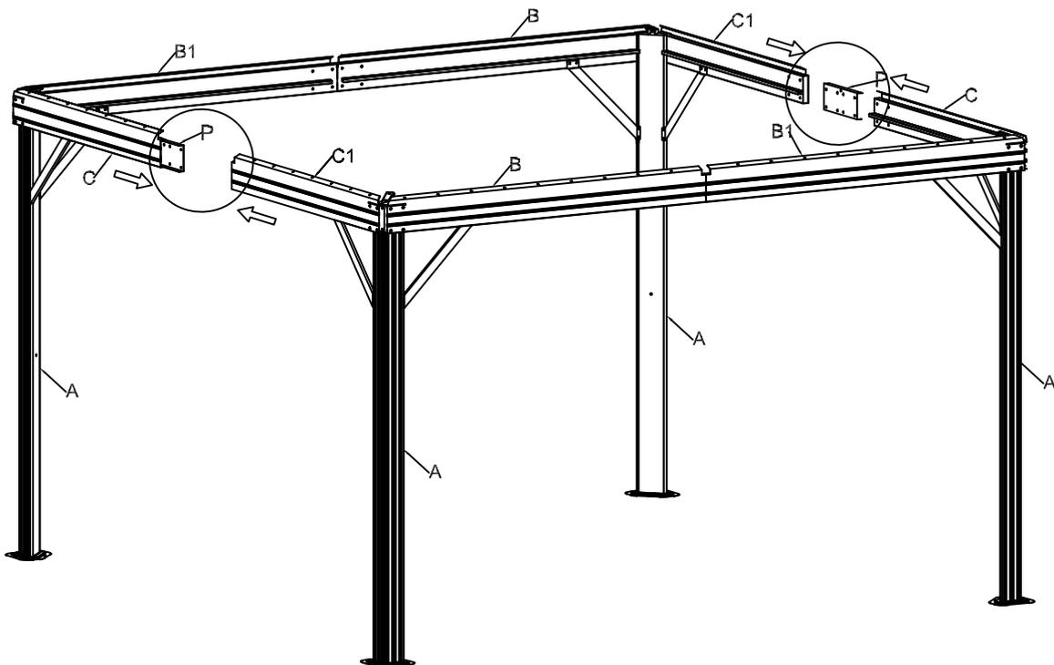
Attach assembled Short Side Left Beam (C) & Short Side Right Beam (C1) to Beam Connector (P), fix by using Bolt (X1)
