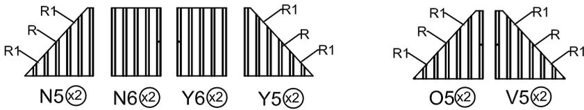
attach the clips(R1) and clips(R) as shown in the diagram
