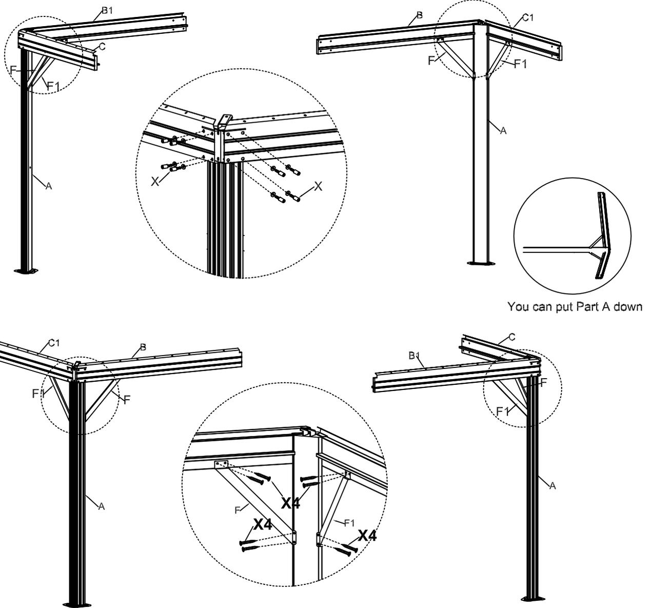
1-Attach Long Side Beam (B/B1) and Short Side Beam (C/C1) to Post (A), fix by using Bolt (X).
