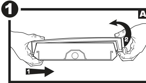
**A** Remove diffuser from housing by sliding diffuser to one side, then lift up opposite side over flange as shown.
