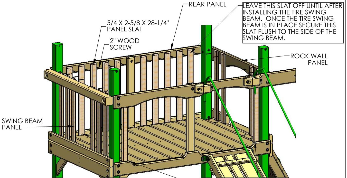
LEAVE THIS SLAT OFF UNTIL AFTER INSTALLING THE TIRE SWING BEAM. ONCE THE TIRE SWING BEAM IS IN PLACE SECURE THIS SLAT FLUSH TO THE SIDE OF THE SWING BEAM.
