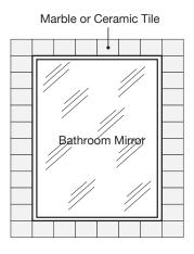
Lack of gaps in the mirror and hard objects such as a tile or marble close to the heated mirror may cause a crack as they cannot expand freely if a 2mm gap is not left.
