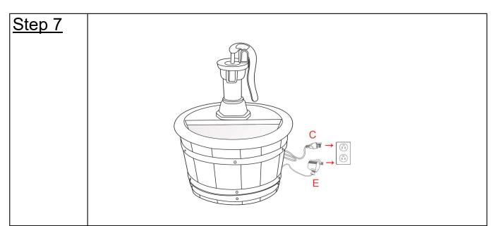
Plug the Pump(C) and Transformer(E) in the socket, then the water will start to flow in minutes.
