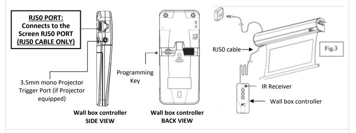
4. Wired 5-12 volt trigger: Requires a 3.5mm to 3.5mm mono cable (not included)
