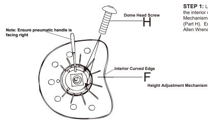
**STEP 1:** Lay the Tractor Seat face down on a soft clean surface with the interior curved edge toward you. Attach the Height Adjustment Mechanism (Part F) to the Tractor Seat using (2) Dome Head Screws (Part H). Ensure mechanism handle is facing right. Tighten with the Allen Wrench (Part I)
