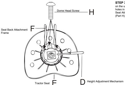
STEP 3: Place the Seat Back Attachment Frame (Part F) on the underside of the Tractor Seat (Part E) on top of the holes in the Height Adjustment Mechanism. Attach the Seat Attachment Bracket using (3) Dome Head Screws (Part H). Tighten with the Allen Wrench (Part I)
