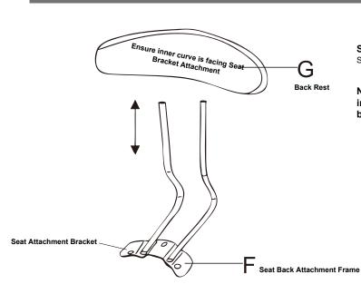
**STEP 2:** Push Seat Back (Part G) onto posts of Seat Back Attachment Frame (Part F).
