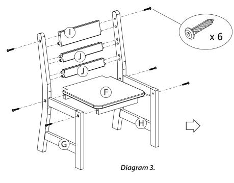
Assemble chair by attaching Seat (F), Chair Left Frame (G), Top Back Rest (I), Middle Back Rest (J) and Chair Right Frame (H) together by using 6 Screws JCA 1/4" x 38 mm as per diagram 3.
